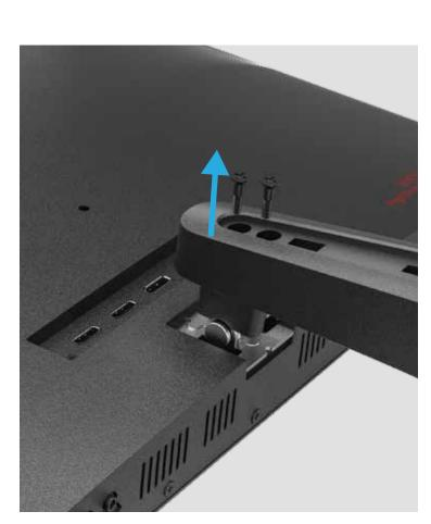
Using a Phillips screwdriver Take out the base. remove the screws.
